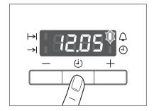
2. Using the + or — button set the desired Countdown (max. 2 hours 30 minutes).
